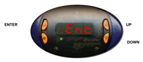
To enter set-up mode, hold the Enter and Down buttons together for approximately 3 seconds until the message "Ent" appears on the display. Now press the Enter button again to enter the function menu. IO will be displayed. Scroll up or down to go through the list.
